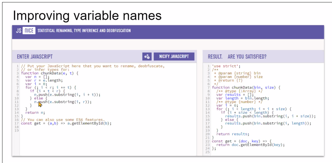
Figure 38: JS Nice tool, browser interface for renaming, type inference, and deobfuscation.
